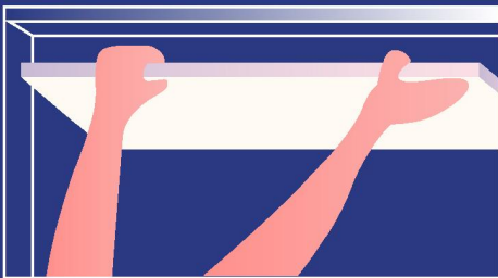
01 Hang the PowerBoard on the suspended ceiling profiles
